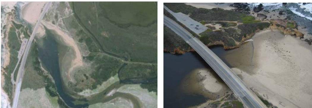
Figure 6 – Aerial images of Pescadero mouth on 19 May 2007. Note the lobe of sand extending landward under the Hwy-1 Bridge as a subsurface flood-shoal. Photos courtesy of Rusty Holleman.
