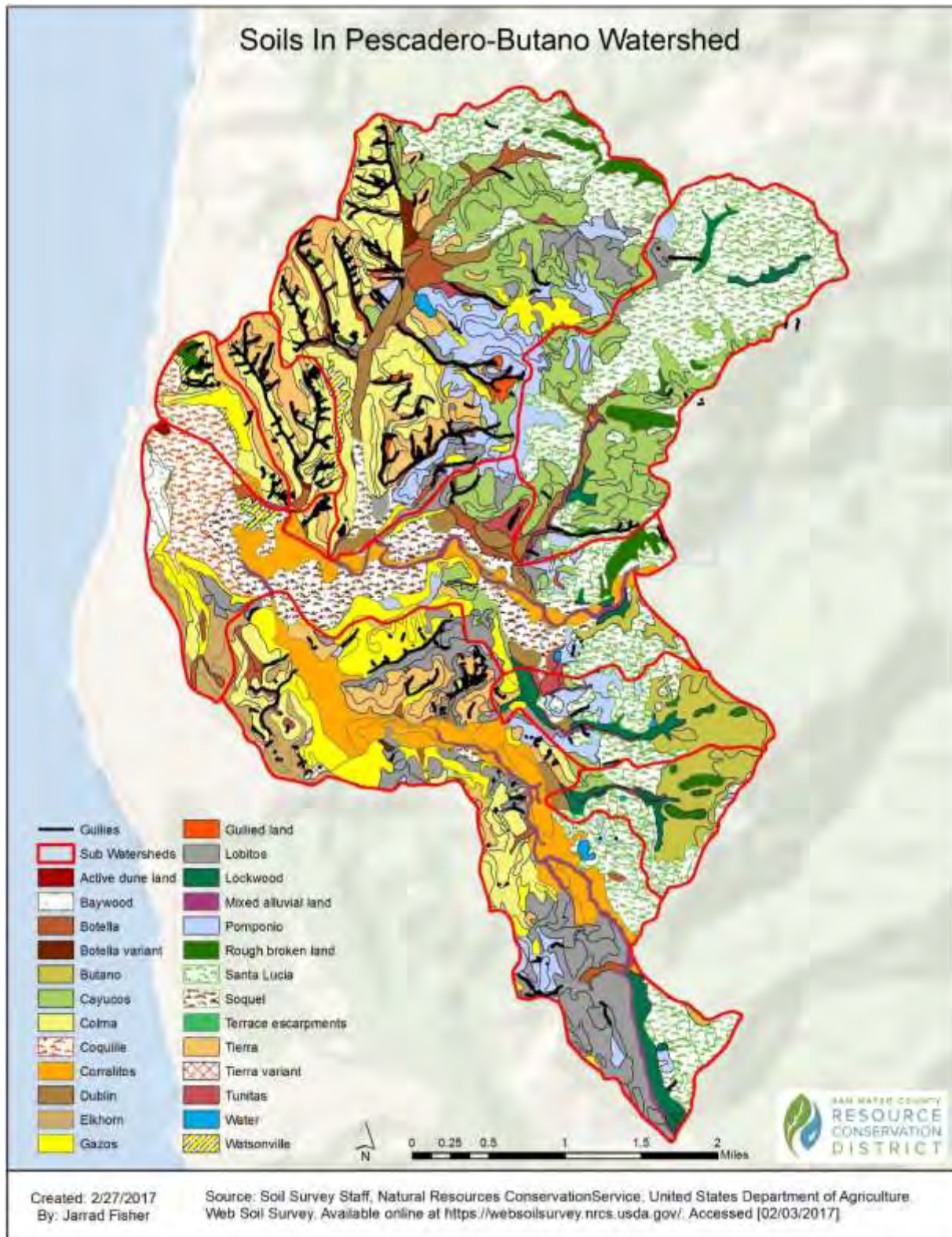
Figure 20. Locations of gullies (RWQCB 2012) in the lower PBW with respect to soil type. Gullies in the northwest subwatersheds (i.e., Tributaries 1 and 2, and Bradley) are primarily found in the Tierra and Colma soil types. In the Lower Butano subwatershed, gullies occur on Tierra, Colma, Lobitos and Gazos soil types.
