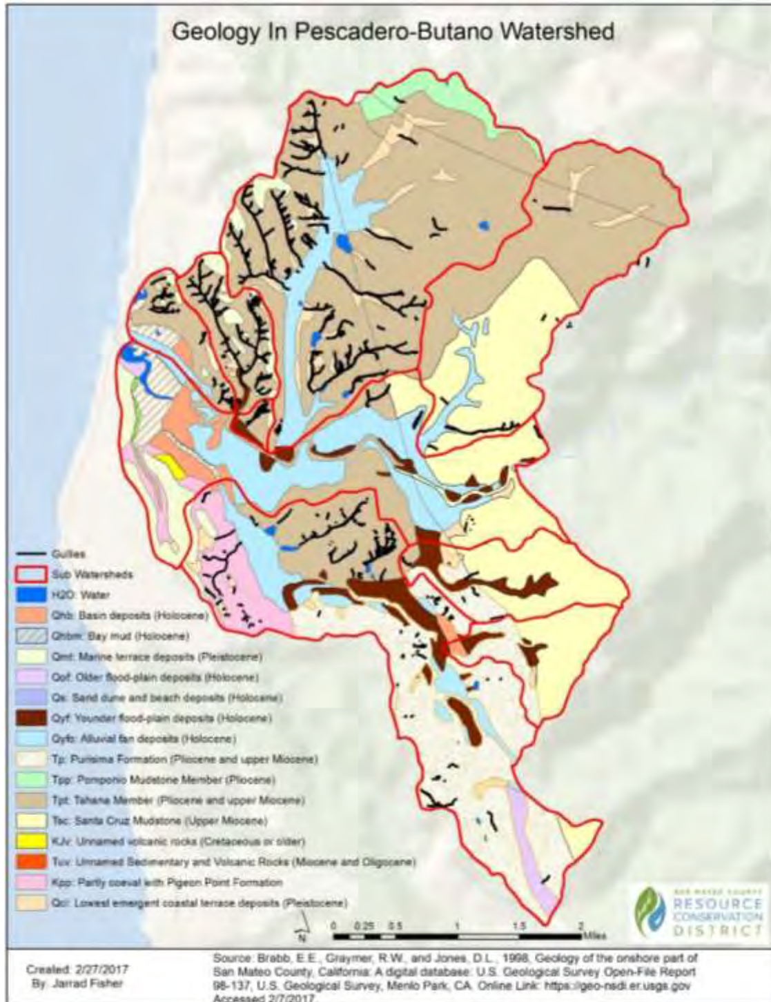
Figure 19. Locations of gullies (RWQCB 2012) in the lower PBW relative to geologic unit. Gully networks are common over the Purisima Formation Tahana Member (Tpt). Shorter, less developed networks are present on the undifferentiated Purisima formation (Tp) and Pigeon Point Formation (Kpp). One notable large gully is seen in the Santa Cruz mudstone (Tsc). Gullying over the Tahana appears concentrated in the coastal portion of this formation within the study area, and decreases further inland.
