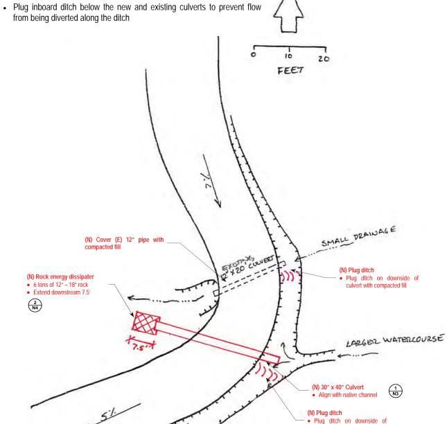
culvert with compacted fill
