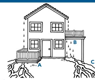
A Low decks may prohibit the addition of protective ground cover, leaving bare soil to erode.
