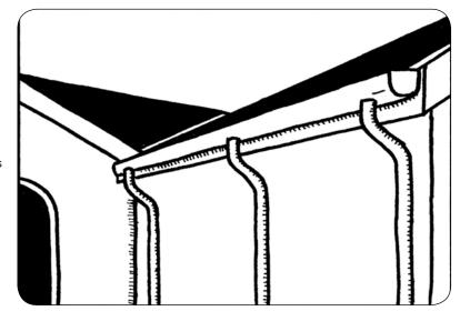
Adding an additional downspout helps reduce the volume and velocity of runoff at any
