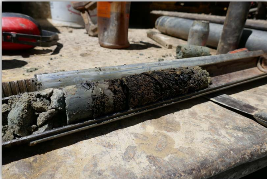
Photo 6 Photo of the core sample taken near the end of Boring B1. The photo shows the log at the base of the fill (to the right) on top of sandstone bedrock (to the left)
