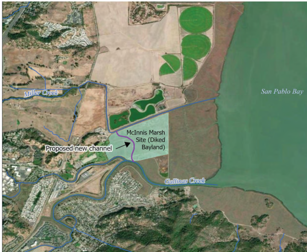
Figure 21. Proposed realignment of Miller Creek to flow into Gallinas Creek at McInnis Marsh (adapted from KHE 2016). This provides a high-level concept view only; actual design would include more tidal channels.
