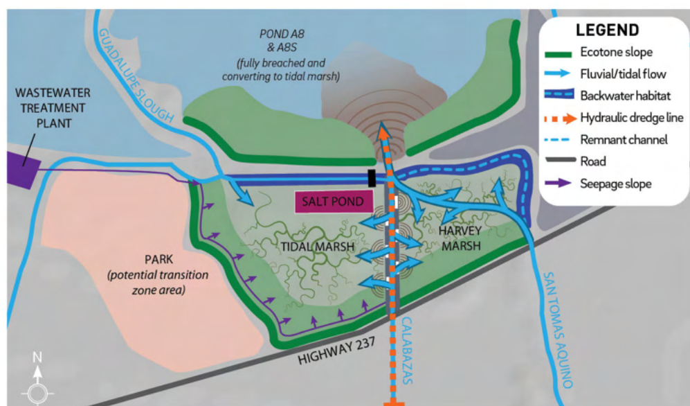
Figure 20. Planning documents envision Calabazas and San Tomas Aquino Creeks to flow directly into Pond A8 by realigning the creeks via a breach through the existing levee and creating off-channel reconnections, which will be discussed in the next section, between Calabazas Creek and Harvey Marsh (McKnight et al. 2018).
