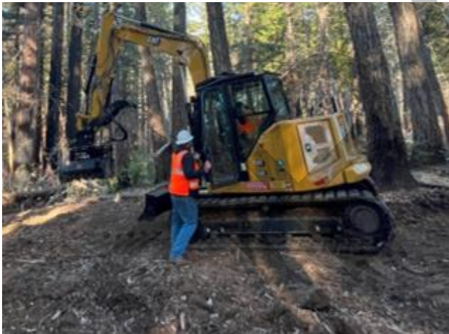
Figure 2. Examples of Mechanical Equipment – Cat 308 excavator with masticating head attachment (left). Cat 299 skid steer with grapple attachment (right).
